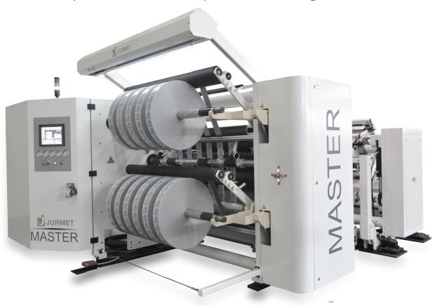
High performance machines for slitting and rewinding flexible materials with possibility to integrate punching / laser unit or Work Flow solutions
